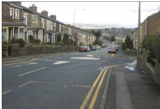
Photo 3.3.1: Constrained site where all vehicles from side road have to overrun central island
